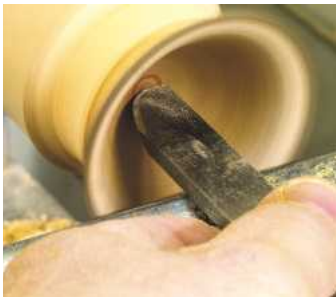
▲ Pic.5 If you want to you can finish the inside curve off with a French curve scraper, taking light cuts and watching that edge – you don't want to knock it off now
